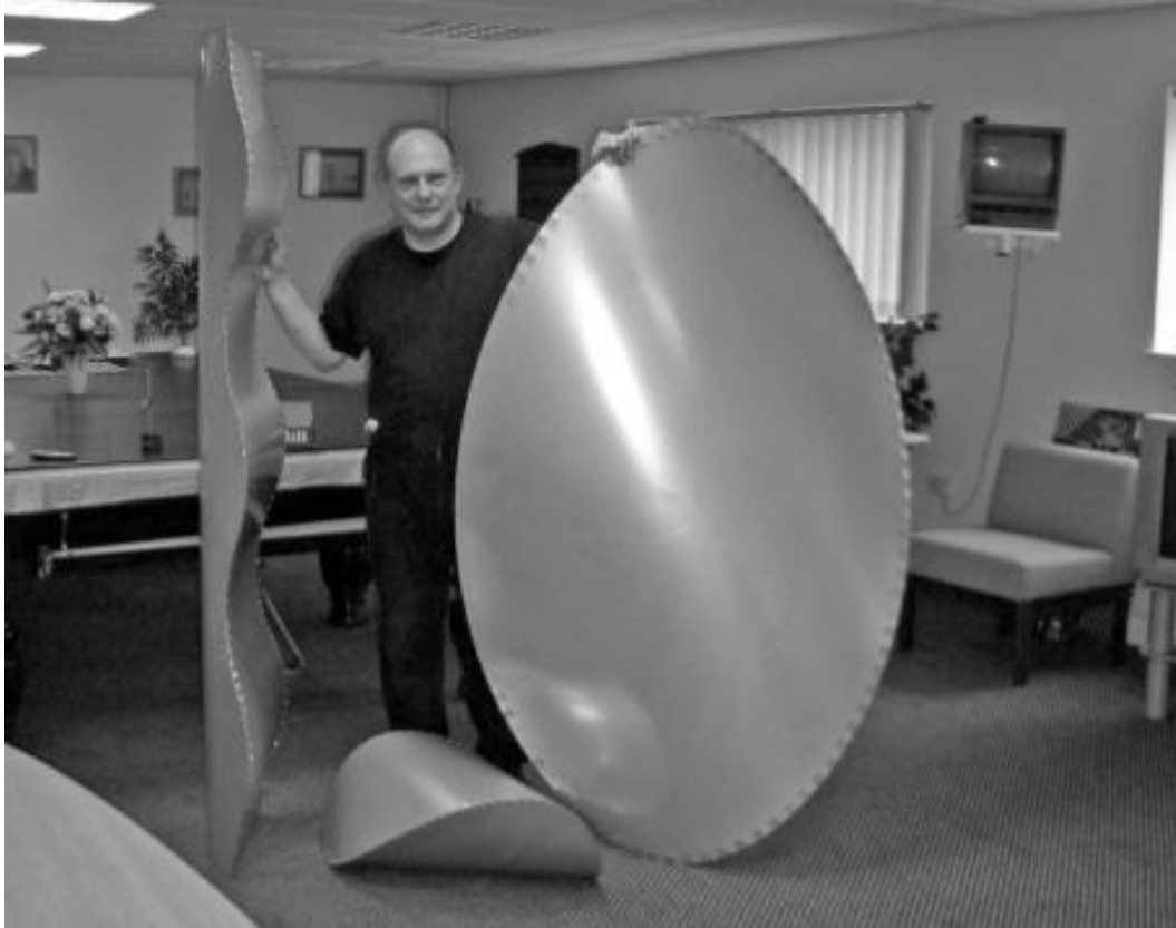
Figure 7, D-Forms made from sheet steel (held by Tony Wills).
