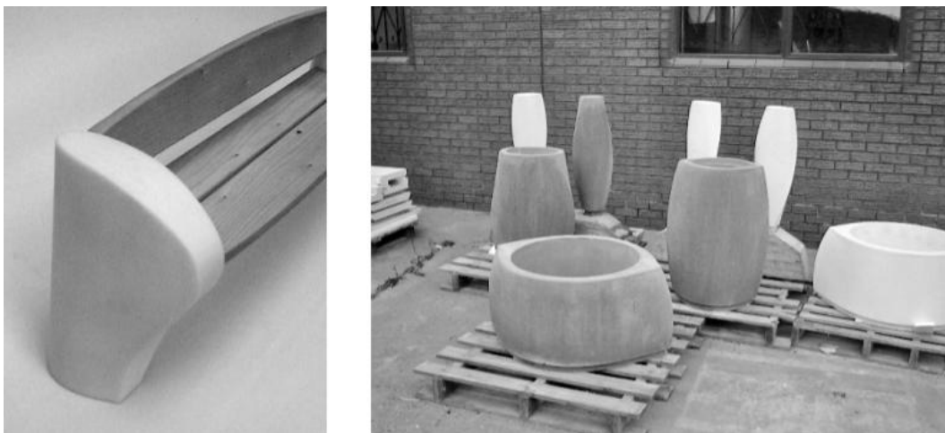
Figure 8 shows how D-Forms have been used as part of a bench. The ends of the bench are cast in concrete using a D-Form.
