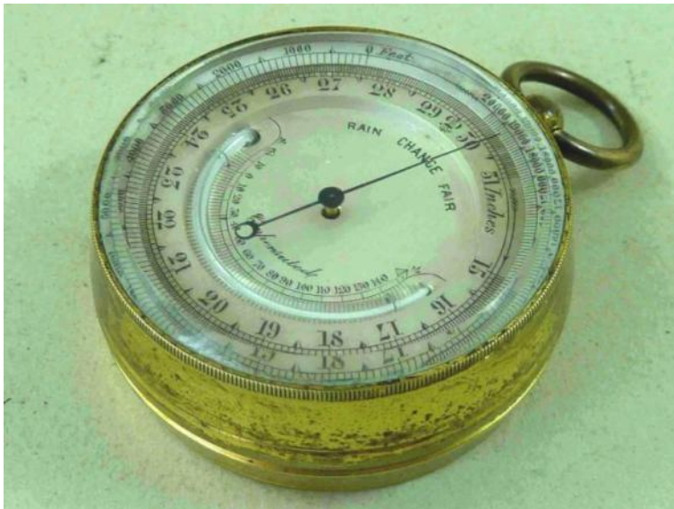
A 19th Century barometer and altimeter, of the type used by David Wedderburn for measuring height above sea level.
