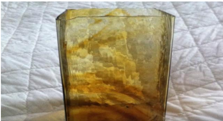
This is a piece of Norman Slab where the sides have not yet been broken out.
