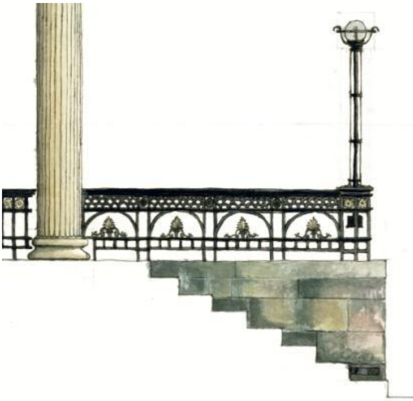
'1:20 Scale Section Study of Entrance Steps at no.8 Great Western Terrace', By Will Knight.
