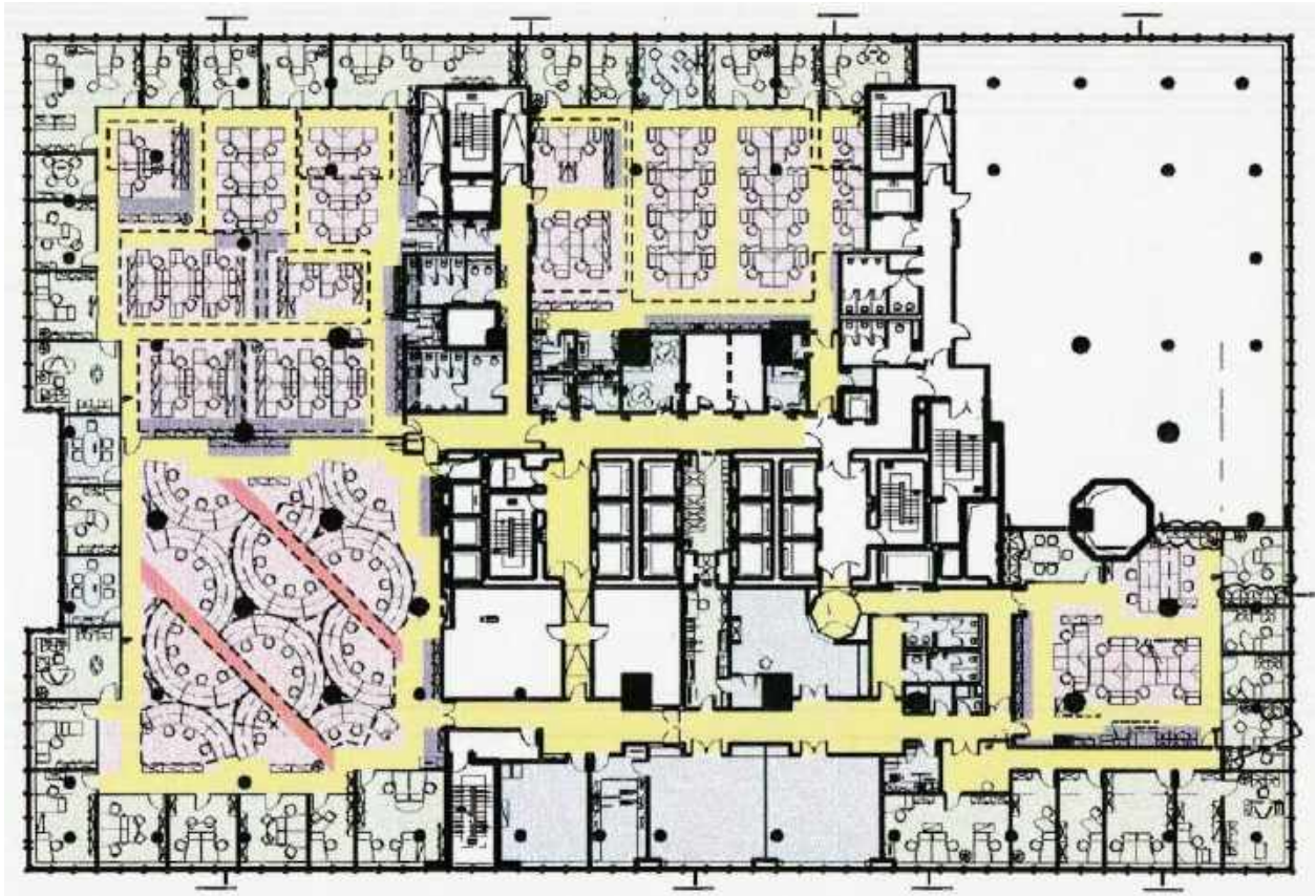
Eurotower, Frankfurt, Salomon Brothers layout for move-in 1996, with curved trading desk groups.
