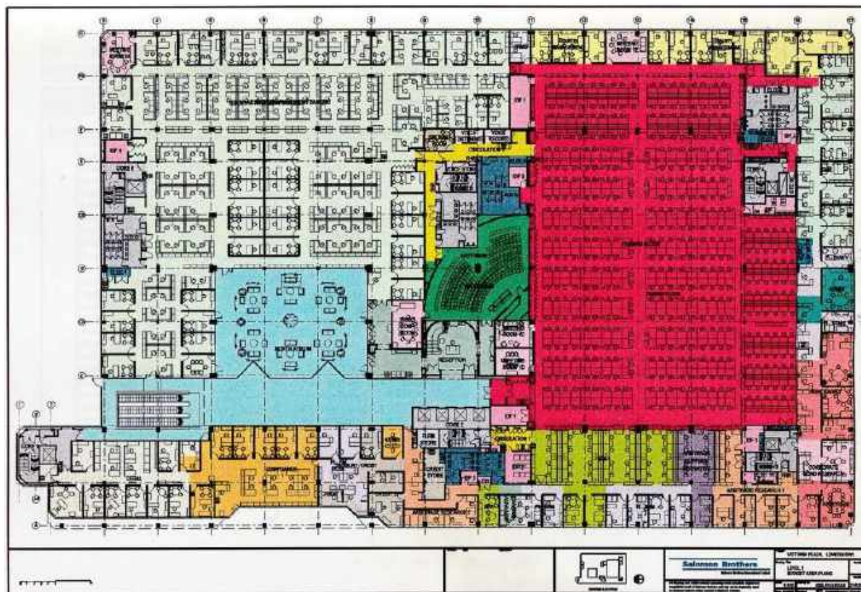
Victoria Plaza - Level 1 showing trading floor (red) surrounded by research and managers. Investment banking (left hand side). (Reduced) North atrium area in blue with escalators to ground level.
