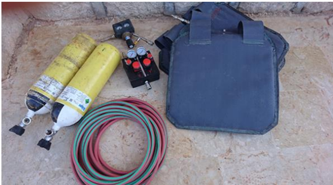
Field Ready Rescue Airbag Kit: regulator, valves, compressed gas tanks and set of two airbags. Credit: Field Ready.
