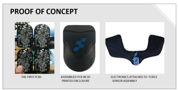
We sourced cables, connectors and components. We got our first custom circuit boards made and assembled. Another friend 3D printed us some enclosures which we spray painted black and then used Sugru to emboss the logo. We built our sensor assembly and encased the sensors in protective EVA foam, and bound the edges with nylon ribbon. We got a special shirt custom made to hold the sensor assembly while on the player's body. We even made a display box, which ended up looking like a pizza box.
