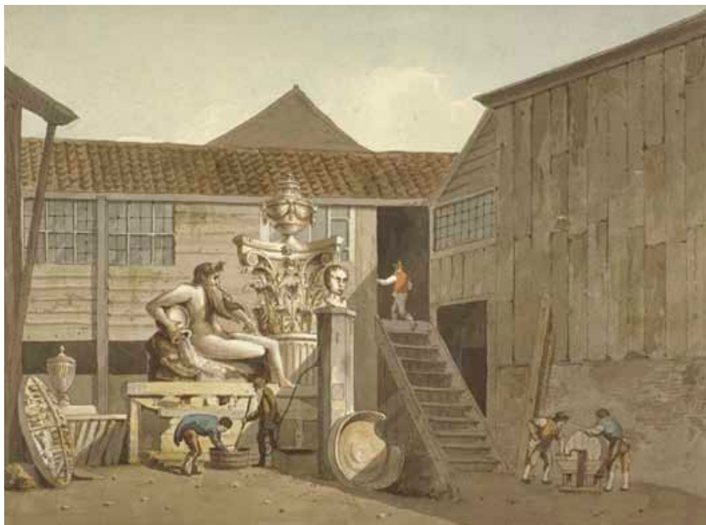
Fig. 3. The yard at the Coade manufactory, c.1804. John Bacon's River God features prominently; workmen are grinding the ceramic's constituents ( London Metropolitan Archives, City of London )
