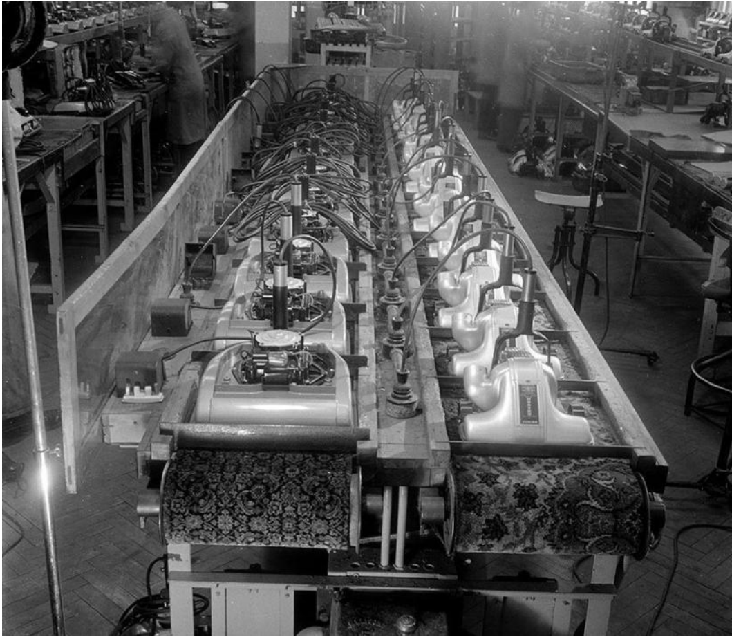
Testing hoovers on a rolling carpet device at the Hoover factory, Perivale, 1948. Walter Nurnberg/Science Museum Group Collection.
