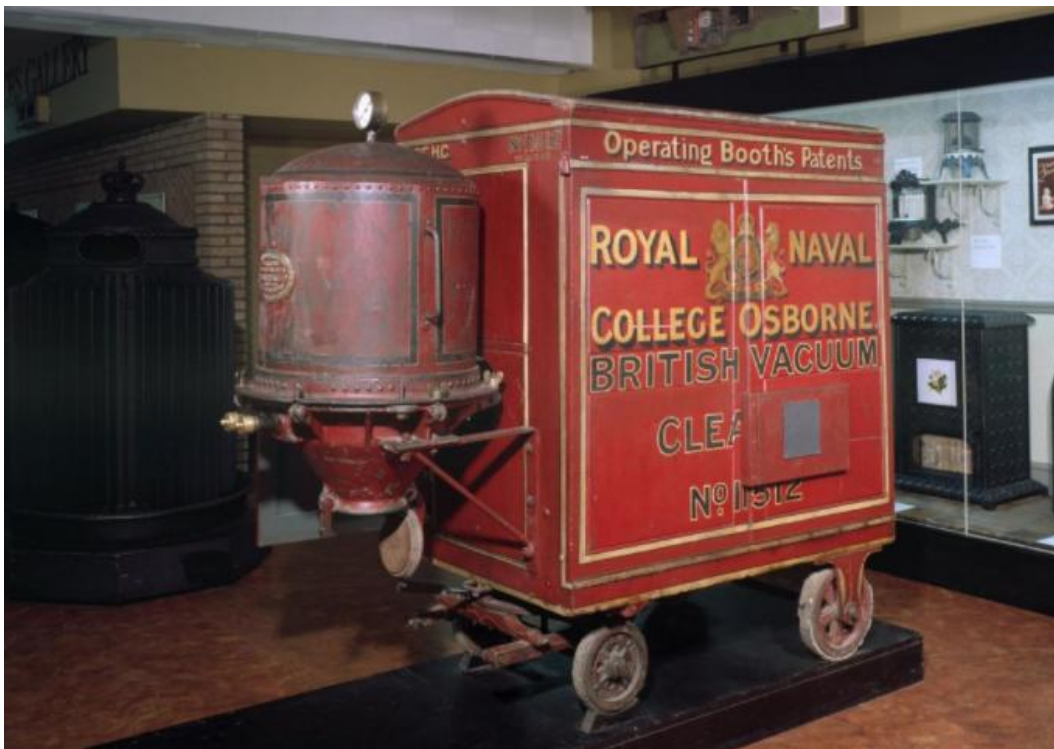
Original Booth trolley vacuum cleaner, supplied to the Royal Naval College, Osborne, c.1905. Science Museum Group Collection.
