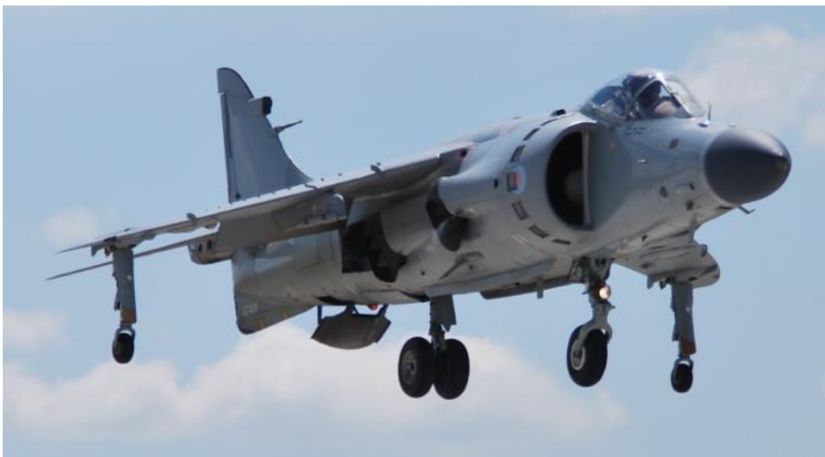
The Sea Harrier was a vertical take-off and landing (VTOL) naval jet fighter.
